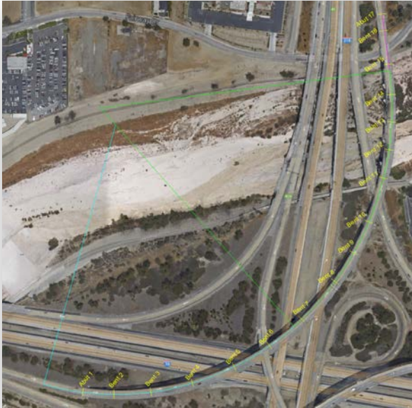
Determination of curve superelevation at each sampling point
